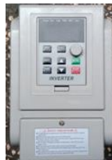
Gambar 3. Inverter VSD AT1.
