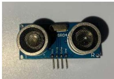
*Gambar 1. Sensor Ultrasonik*
