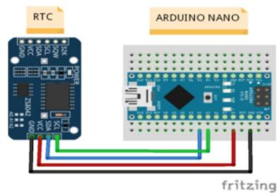
**Gambar 4.3** Skema Rangkaian RTC (*Real Time Clock*).
