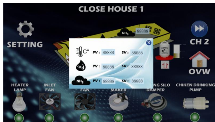
Gambar 18. Close house setting
