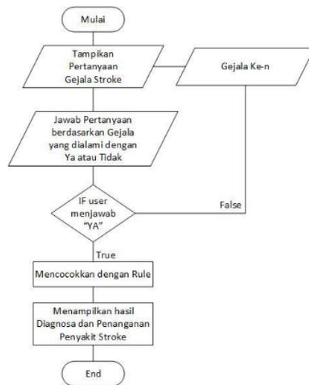
**Gambar 1.** Mekanisme Metode Forward Chaining
