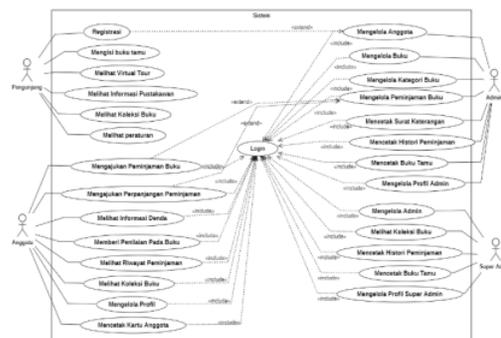
Gambar 4.2 Use Case Diagram
