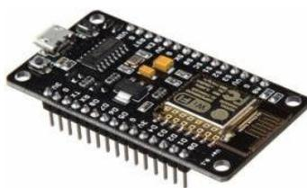
**Gambar 1. NodeMCU ESP8266**
