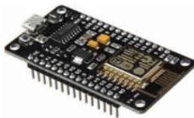
**Gambar 1. NodeMCU ESP8266**
