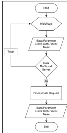
**Gambar 3. Flowchart pengambilan data dikirim ke server via LoRa**
