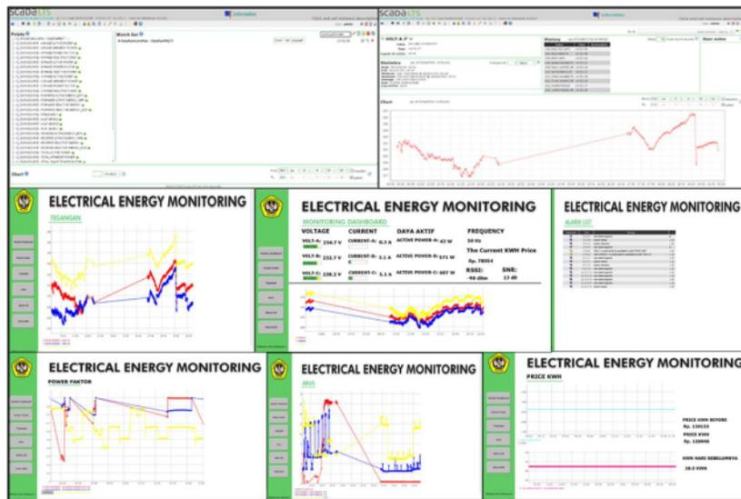
**Gambar 6. Desain Scada-LTS**
