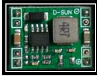
**Gambar 2.3** Modul *Step Down DC – DC MP1584*
