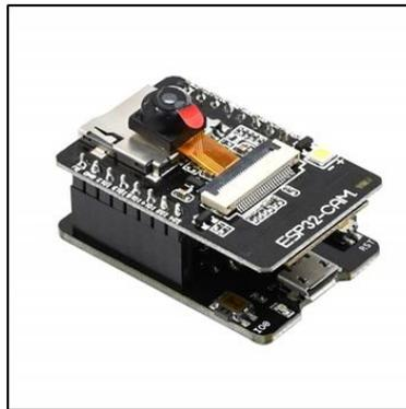
**Gambar 4. ESP-32 CAM**
